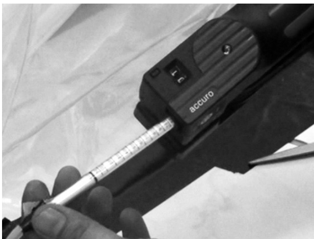
Gambar 2. Accuro Pac 7000, alat pengukur kosentrasi gas phosphine
